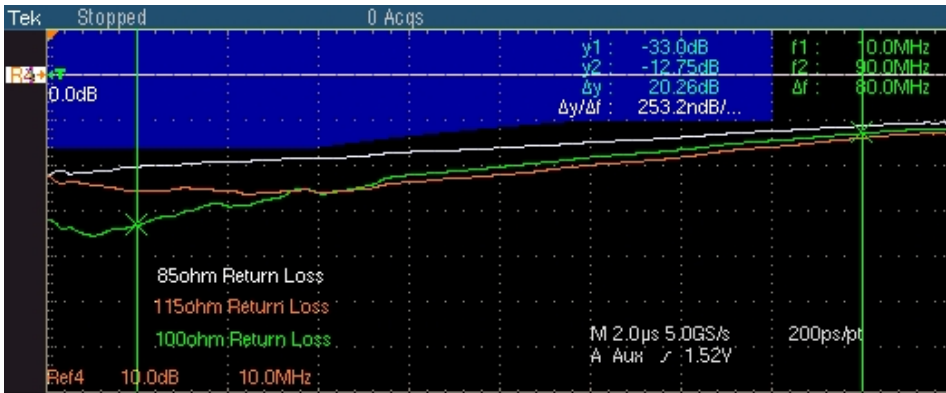
Figure 9-18: Waveform for 100BASE-TX Return Loss Transmitter
